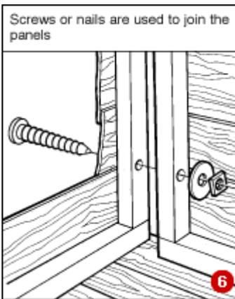
The panels are joined to each other through pre-drilled holes, using screws and washers or nails (6). It is usual to start with a side and back panel, then to add the other side panel, and finish with the door section.
