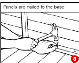
The wall panels are secured to the floor joists using screws or nails (8). If nails, knock them in at an angle (skew nailing).
