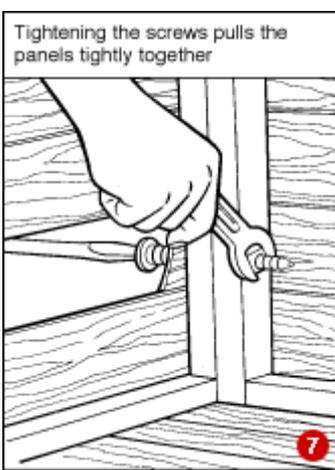
The action of tightening the screws or banging home the nails draws the wall panels together (7). Subsequent panels are secured to each other.
