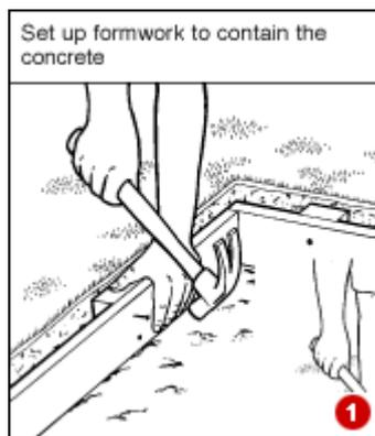
Set up formwork to contain the concrete
